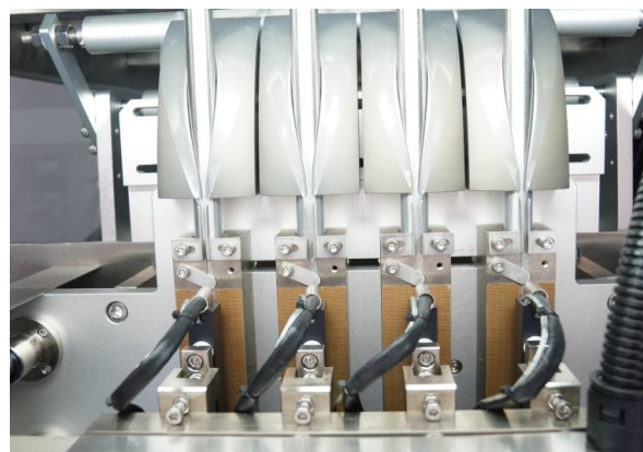
Bag making and forming+longitudinal sealing mechanism
