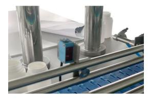
The bottle photoelectric eye will determine whether there is a bottle at the discharge port (no bottle does not work)
