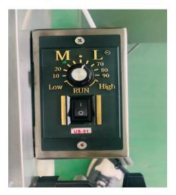
The conveyor belt speed control switch is used to control the speed and start stop of the conveyor belt
