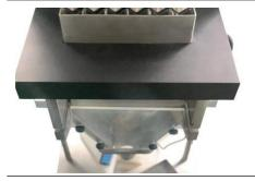
The materials pass through the vibrating plate and fall into the medicine bin by the counting photoelectric system
