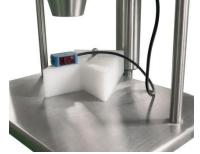
The single discharge port bottle inspection photoelectric eye can determine whether there are bottles at the discharge port (it won't work without bottles).
