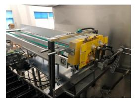
Feeding device: Servo feeding, with optical eye detection. No material does not leave the box, which can avoid empty boxes and waste
