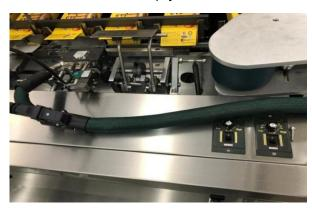
Box sealing device: It can achieve automatic box closing and sealing, and is equipped with a hot melt adhesive machine to make the box flat and more compact and flat after sealing
