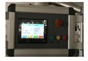
It adopts a human-machine interface operating system, an imported brand touch screen, which is simple to operate, stable and reliable. It is equipped with a PLC automatic control system and variable frequency speed regulation. All electrical components are from internationally renowned brands
