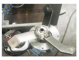
The mixing shaft is fixed on the bearing seat, which is equipped with two sets of bearings
