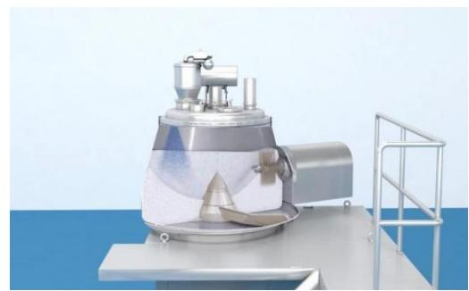
△ Sealing failure alarm: There is a pressure detection at the gas seal of the cutting blade, and the sealing failure system alarms in a chain, stopping the current production state;
