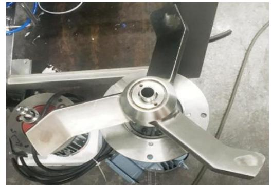
The mixing shaft is fixed on the bearing seat, which is equipped with two sets of bearings corresponding to axial and radial forces on the upper and lower parts of the bearing seat. The working torque of the motor is reduced, which reduces the pressure on the shaft seal and extends the service life of the shaft seal by about 1200 hours;
