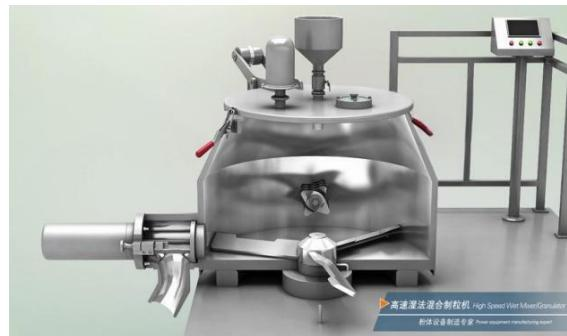
2. The GHL series high-efficiency wet mixing granulator adopts a horizontal drum structure and advanced design.
