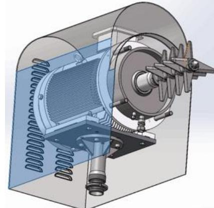
△ Variable frequency speed regulation: The cutting blade motor adopts a stainless steel outer cover, and the cutting blade speed is variable frequency regulated on the touch screen display.
