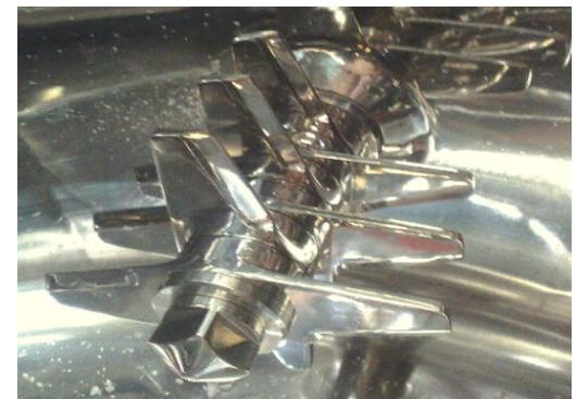
The Z-shaped blade design is more conducive to the flipping of materials and the effect of explosive flow rate compared to the old-fashioned blade design;
