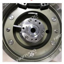
The filling base adopts a negative pressure design, which can suck the powder in the hole of the base through negative pressure when the equipment is running, and recycle it into the powder collector. Effectively avoid the waste and loss of the powder, and realize the secondary use of the powder.
