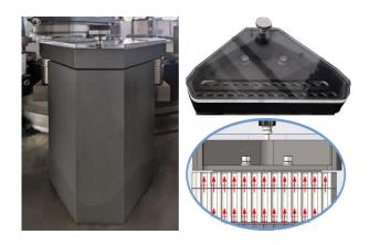
Purified compressed air and intermittent gas impingement technology are adopted. It solves the problem of powder sticking to the mold and improves the probability of capsule loading.
