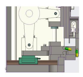
Driven by guide rail, it has high precision and long service life. The closed design effectively prevents waste capsules and dust from entering. Good stability, orderly seeding, and accurate direction adjustment.
