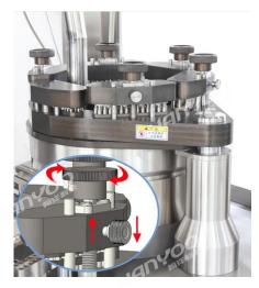
Modular design is adopted, and the pin-type positioning of the filling holder is used. During production, there is no need to stop the machine to adjust the filling capacity, and it is convenient to replace different filling rods.
