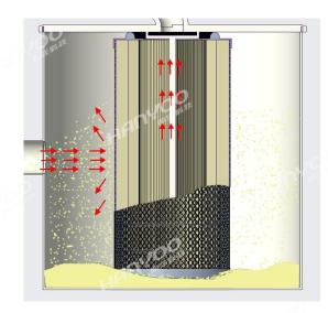
Negative pressure technology is adopted, and it is equipped with an independent distribution system for powder, which can accurately recover powder and avoid crossover Pollution, the recovered powder can be directly produced again, which is convenient and efficient.
