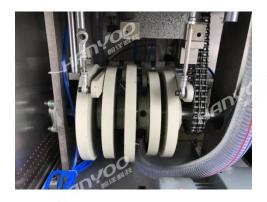
Adopt the latest cam bottom transmission system, the transmission bracket runs through the top and bottom of the design, all the running cams use inner groove cams instead of honest outer cams, and the high-speed operation achieves precision, accuracy, stability and no noise.
