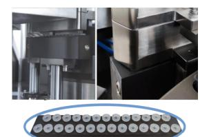
A soft sealing column is installed on the original suction seat, and the balance between the lower mold and the suction seat is automatically adjusted by the soft sealing column during the production process to prevent vacuum leakage and increase the rate of capsule separation.
