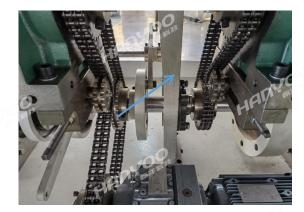
Adopt the latest cam bottom transmission system, the transmission bracket runs through the top and bottom of the design, all the running cams use inner groove cams instead of honest outer cams, and the high-speed operation achieves precision, accuracy, stability and no noise.
