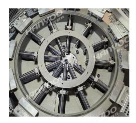
The frame of the 12-station turntable adopts one-piece processing, which has a compact structure and no splicing gaps, and has good sealing and easy disassembly; the upper and lower modules move independently, and the shaft seal of the fixed bracket adopts a double-lip skeleton dust-proof ring to achieve No noise, small size, small load, high precision. The interior of the fully enclosed rotary table is free of maintenance, oil, maintenance and powder for three years.
