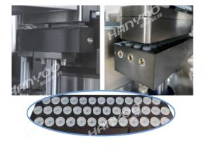
A soft sealing column is installed on the original suction seat, and the balance between the lower mold and the suction seat is automatically adjusted by the soft sealing column during the production process to prevent vacuum leakage and increase the rate of capsule separation.
