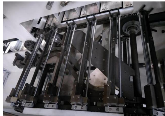
Multiple Pusher(push product into carton box) It' s in the back of the machine,so it' s safer and more convenient.
